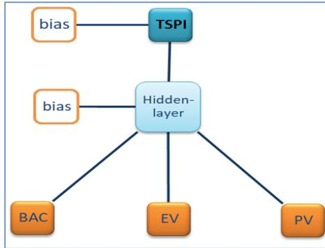
Figure 5. Architecture of TCSPi-ANN Model
