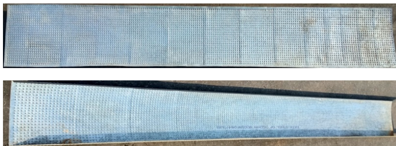
Figure 3: Photograph of one and three sides roughened absorber plates.
