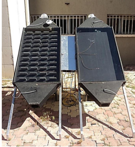
Figure 16: Photographic view of SAHs.
