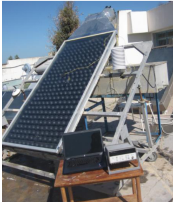
Figure 14: Photographic view of packed bed SAH using PCM spherical capsules.
