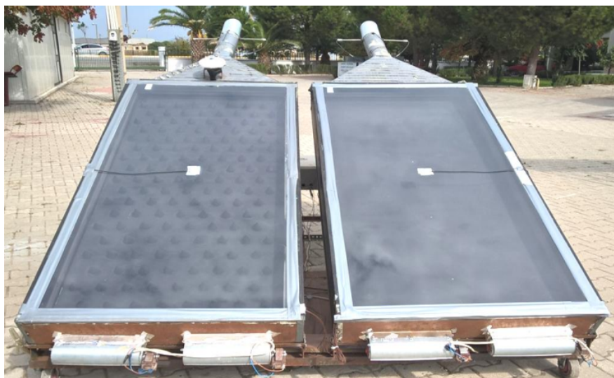
Figure 22: Photographic view of absorber plates with conical surface and smooth SAHs.
