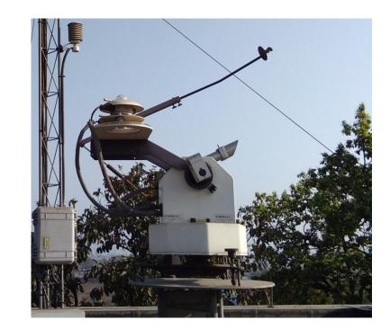
Figure 5: Photographic view of digital pyranometer.
