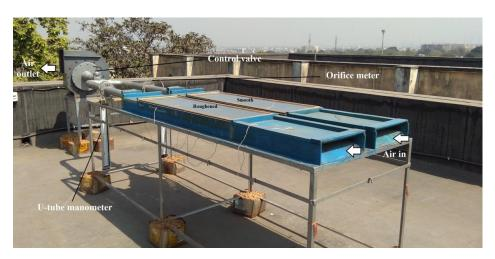
Figure 2: Pictorial view of SAH experimental setup.
