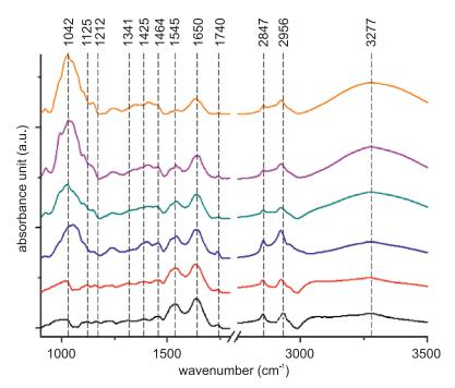
Fig. 1. Average FTIR spectra of honeybees treated with EMF at a frequency of 50 Hz and magnetic induction of 1.6 mT. Control group (black spectrum) and groups treated with EMF for: 2 h (red spectrum), 6 h (blue spectrum), 12 h (green spectrum), 24 h (pink spectrum), 48 h (orange spectrum).
