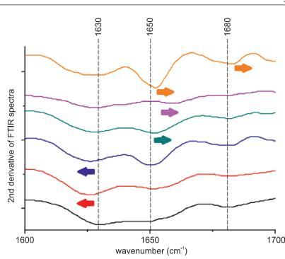
Fig. 2. Second derivative of average FTIR spectra of honeybees treated with EMF at a frequency of 50 Hz and magnetic induction of 1.6 mT. Control group (black spectrum) and groups treated with EMF for: 2 h (red spectrum), 6 h (blue spectrum), 12 h (green spectrum), 24 h (pink spectrum), 48 h (orange spectrum).
