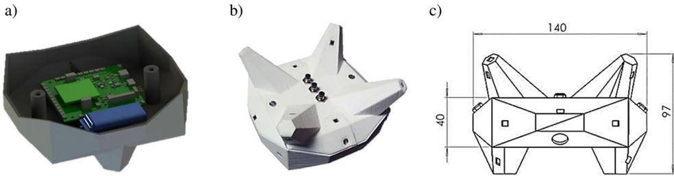
Fig. 4. The lower part of the tracker model prepared for printing: with electronic components (a); photo of the tracker prototype (b) and its dimensions (units – mm) (c).
