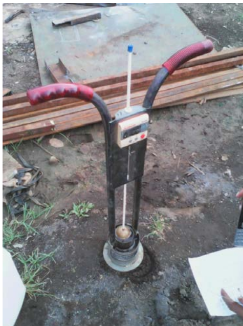
Photo 1. Turf-tec Infiltrometer Model IN2-W (phot. D. Harisuseno)
