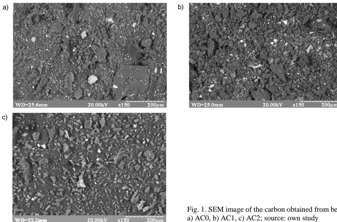
Fig. 1. SEM image of the carbon obtained from beet pulp: a) AC0, b) AC1, c) AC2; source: own study
