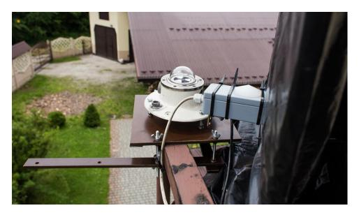
Fig. 3. Eppley solar radiation density meter Source: own study
