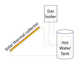
Fig. 6. Scheme of the hot water preparation installation Source: own study based on SHW (UIBK 2017)
