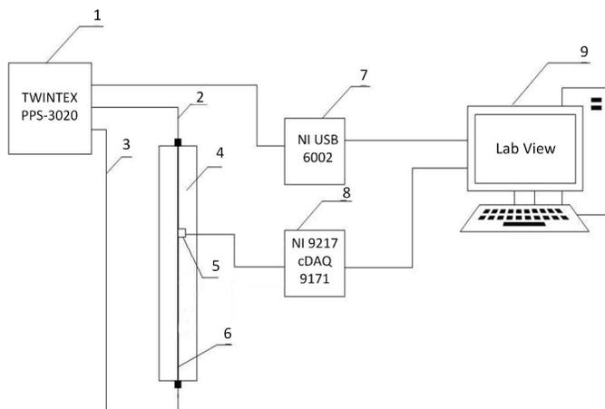
Fig. 2. Experimental set up for measurement of thermal conductivity using the "hot wire" method [25]:
