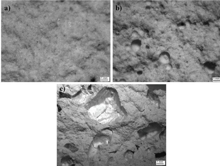
Fig. 3. Microscopic images (magnification  $\times 100$ ) of hardened: a) gypsum, b) gypsum + polymer, c) gypsum + aerogel
