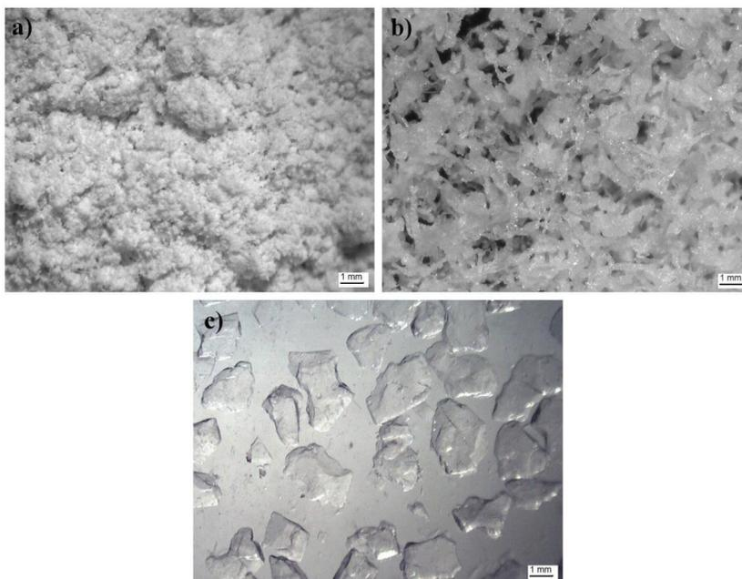
Fig. 1. Microscopic images (magnification x100) of: a) gypsum, b) polymer, c) aerogel
