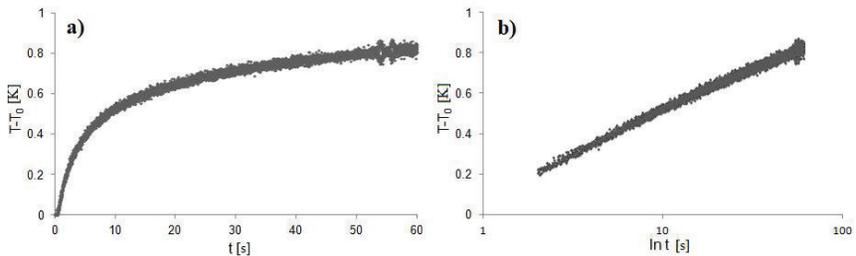
Fig. 4. Graph of the temperature change of the heating wire of the gypsum specimen: a) as a function of time, b) as a function of the natural logarithm of time
