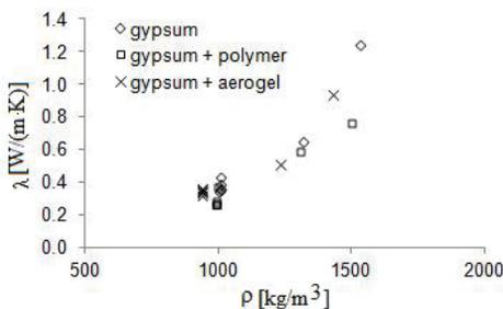
Fig. 6. Graph of the dependence of  $\lambda=f(\rho)$  of the gypsum specimens with different moisture contents
