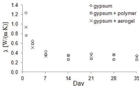
Fig. 5. Changes in thermal conductivity of gypsum specimens during the aging process of the pure gypsum and the gypsum with micro additives
