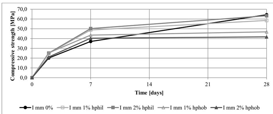
Fig. 3. Development of compressive strength of cement paste with admixture of nanosilica mixed by I mixing method (I mm)
