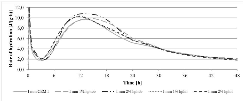
Fig. 1. Hydration heat of cement pastes mixed with a) I mixing method (I mm)
