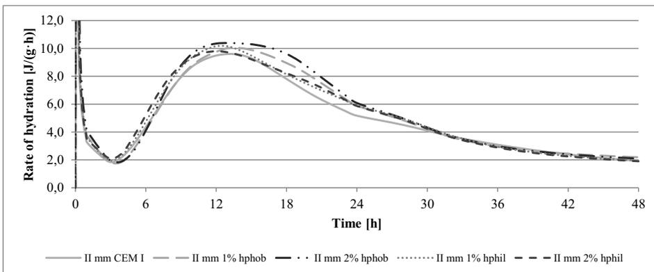
Fig. 2. Hydration heat of cement pastes mixed with b) II mixing method (II mm)
