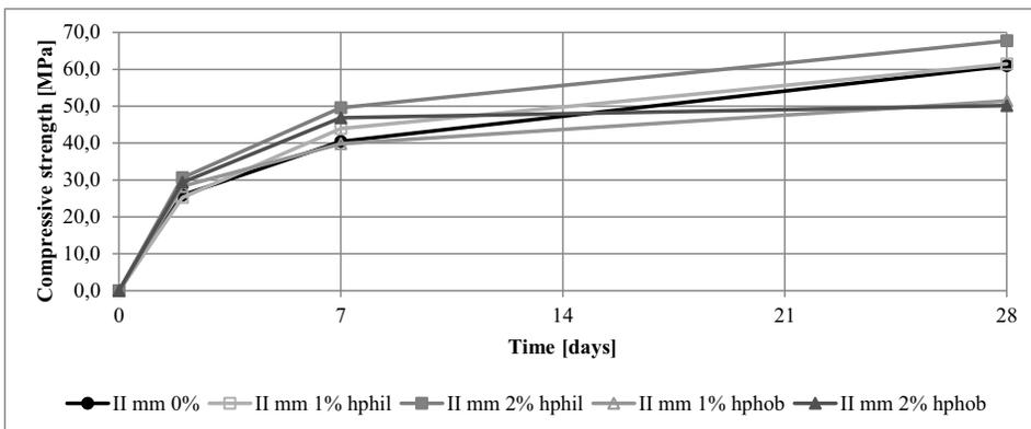
Fig. 4. Development of compressive strength of cement paste with admixture of nanosilica mixed by II mixing method (II mm)
