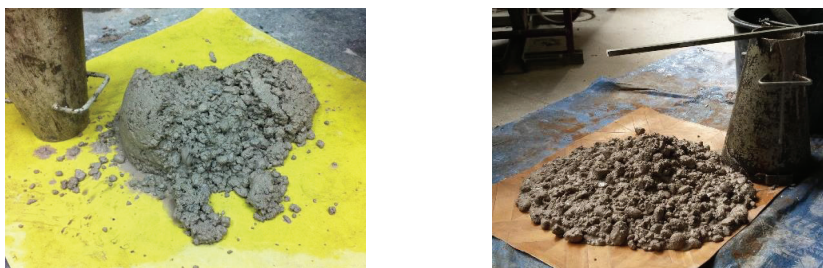
Fig. 1. Concrete mix without (left) and with (right) a superplasticizer
