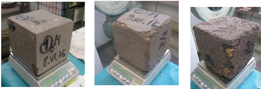
Fig. 6. Sample degradation after 100 freezing/thawing cycles: sample as per recipe No. 1 (left), sample as per recipe No. 3 (centre), sample as per recipe No. 5 (right)
