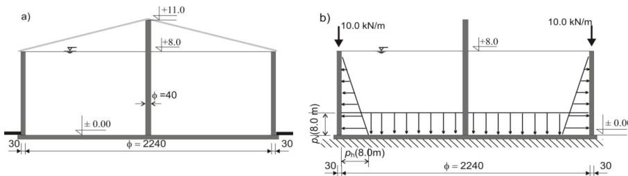
Fig. 3 Analyzed cylindrical tank (dimensions in centimeters): a) vertical cross-section, b) calculation scheme
