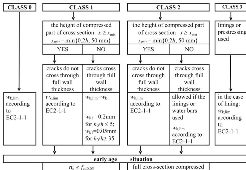
Fig. 1. Liquid tanks classification regarding the tightness according to EC2-3
