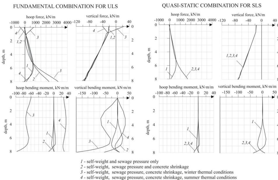
Fig. 5 Comparison of internal forces distributions in different persistent situations: for ultimate limit state and for serviceability limit state
