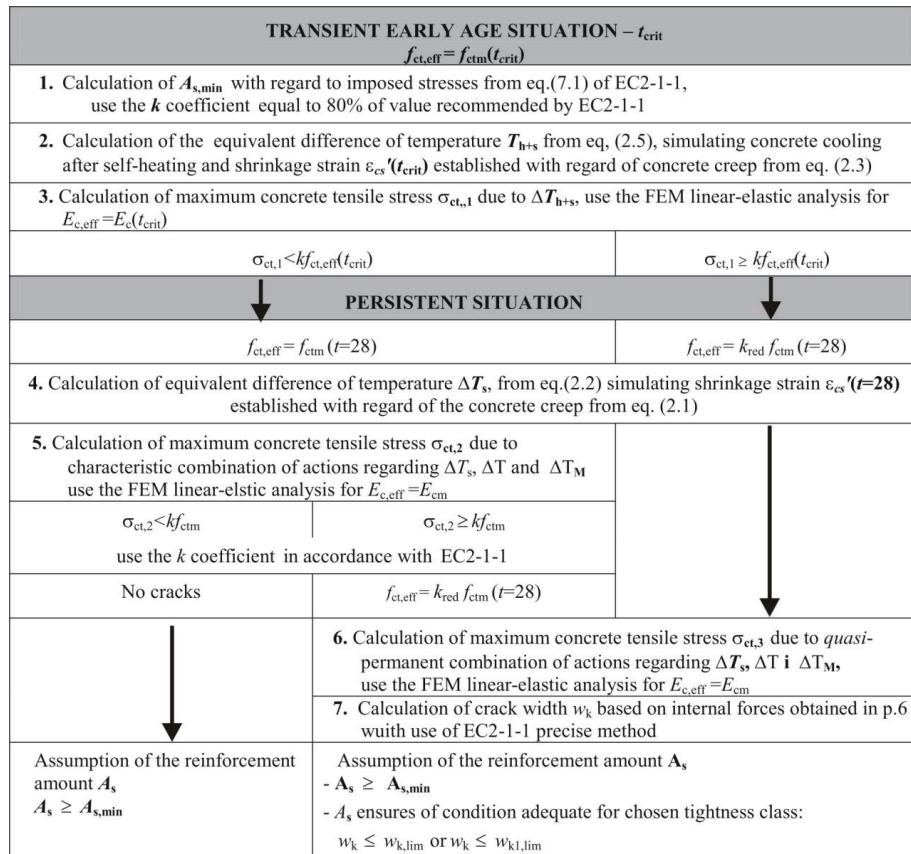
Fig.2 Proposed algorithm for crack control in liquid tank
