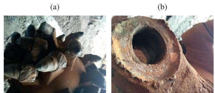
Fig. 1. Worn and broken tooth of the cutting head: a) Worn tooth; b) Broken tooth
