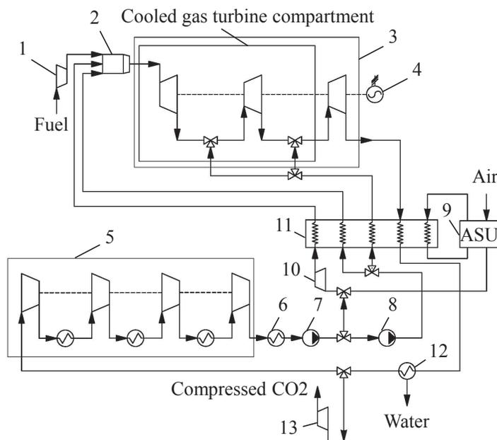
Figure 1: Scheme of the NetPower cycle.
