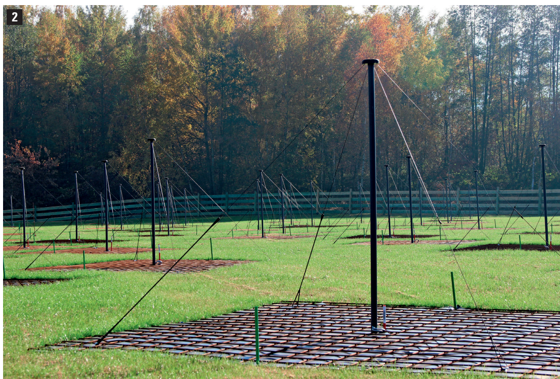
Fig. 1 The Superterp, the heart of the LOFAR core: six separate interferometer stations situated on an artificial island 320 m across. A further 18 stations are situated within a radius of 2 km, and another 14 within the whole of the Netherlands. There are a further 14 international stations (including three in Poland) and that number is continually increasing
