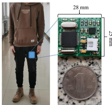
Fig. 2. The wearable device is worn on the thigh, its prototype and size.
