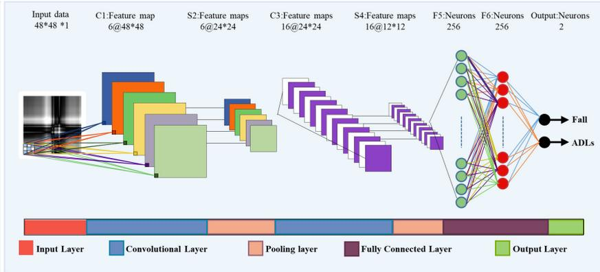
Fig. 7. Architecture of the CNN-based fall detection algorithm at the ML stage.
