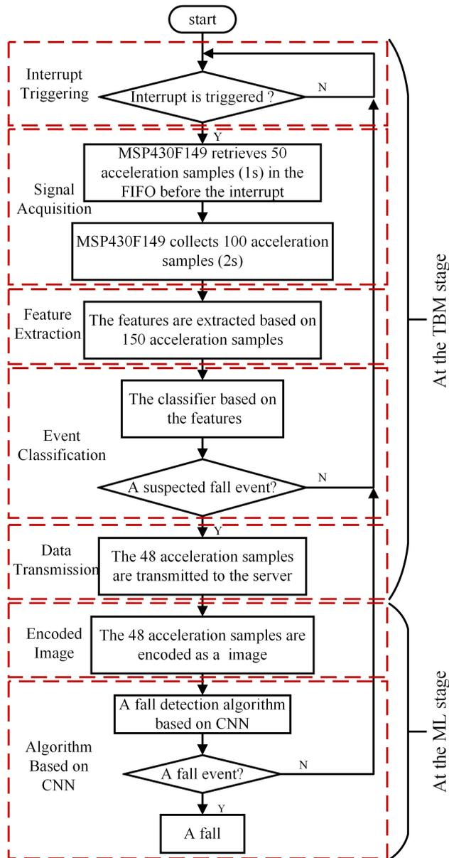
Fig. 3. Flowchart of the two-step fall detection algorithm, including the TBM stage and the ML stage.
