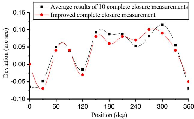
Fig. 3. The position error of the angle comparator.
