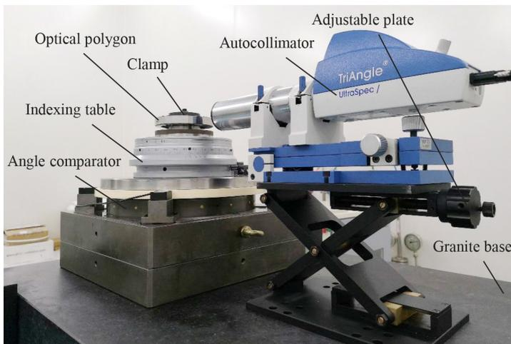
Fig. 1. Arrangement of main devices of the calibration system.
