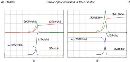
Fig. 7. Voltage waveforms in the transistor, collector and emitter, transistor current, power and energy losses: (a) with a dc-link of 400 V voltage; (b) with a dc-link of 200 V voltage
