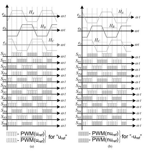
Fig. 6. Waveforms of BEMF, rotor position signals, and transistor control pulses for both directions of rotation: (a) clockwise CW and (b) counterclockwise CCW
