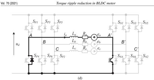
Fig. 4. Path of current flow during one switching period
