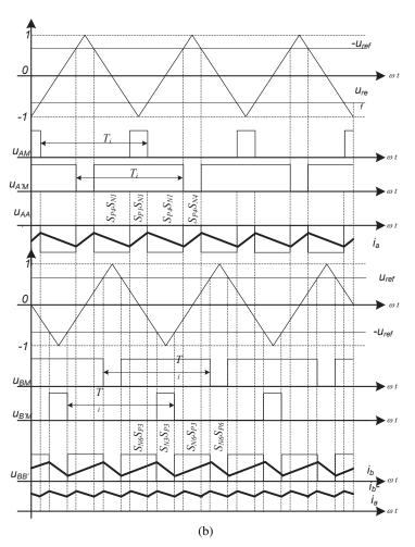
Fig. 2. Method for generating the PWM signal for current flow: (a) from point A to A' and from B' to B; (b) from point A' to A and from B to B'
