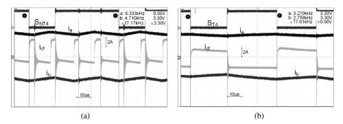
Fig. 13. Waveforms of current for two motor phases, capacitor current  $(i_{cf})$ , pulses controlling one of the transistors with power supply: (a) as in Fig. 1; (b) from a bridge power inverter typical for BLDC motors with unipolar modulation
