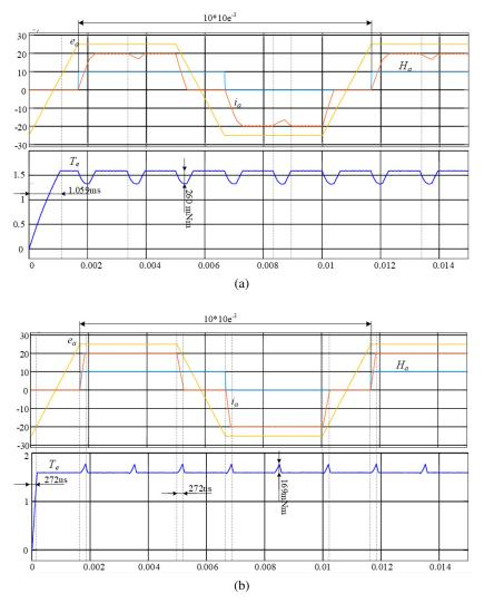
Fig. 9. Waveforms of the current of a single motor phase, back EMF, position sensor and electromagnetic torque signal recorded for: (a) the classic unipolar modulation; (b) proposed solution
