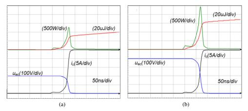
Fig. 8. Voltage waveforms in the transistor, collector and emitter, transistor current, power and energy losses: (a) with a dc-link of 400 V voltage; (b) with a dc-link of 200 V voltage
