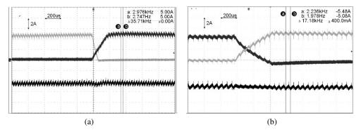
Fig. 12. Current waveforms for three motor phases with power supply: (a) as in Fig. 1; (b) from a bridge power inverter typical for BLDC motors with unipolar modulation
