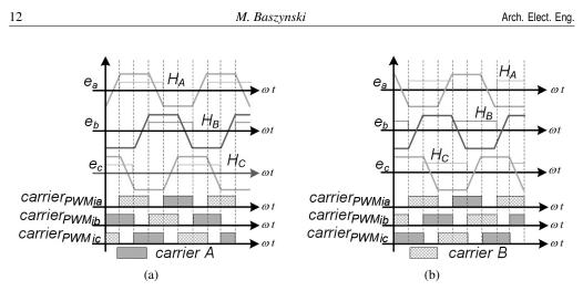
Fig. 5. Assignment of the carrier waveforms to the conducting phases
