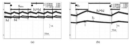
Fig. 14. Waveforms of the absolute value of current for two motor phases, sum of these values, pulses controlling one of the transistors with power supply: (a) as in Fig. 1; (b) from bridge power inverter typical for BLDC motors with unipolar modulation
