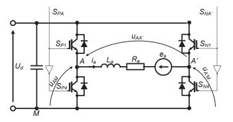
Fig. 3. Marking of the voltages for one phase of the motor
