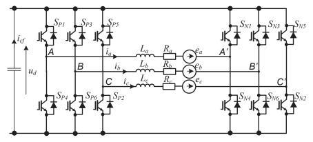
Fig. 1. Open-end winding BLDC motor power supply scheme
