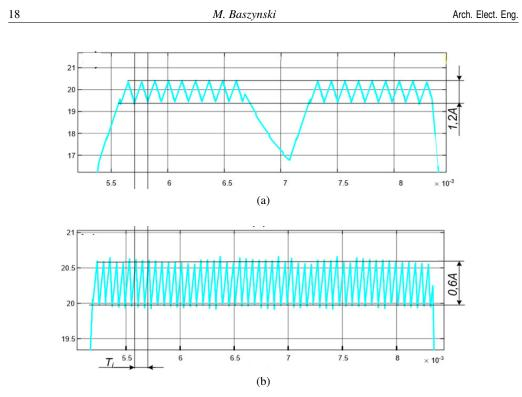
Fig. 10. Zoomed in waveforms of the current of a single motor phase developed for: (a) the classic unipolar modulation; (b) proposed solution
