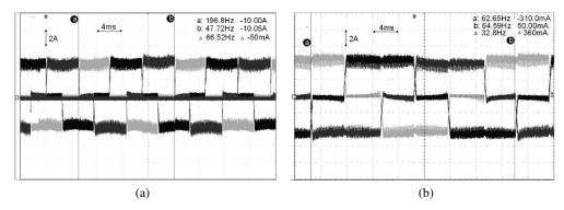
Fig. 11. Current waveforms for three motor phases recorded for: (a) unassociated motor windings powered as in Fig. 1; (b) windings connected in star configuration and supplied from a typical bridge power inverter
