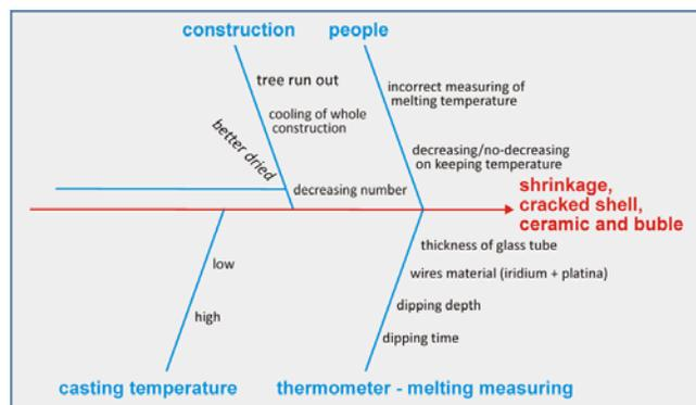
Fig. 3. The cast parts defects demonstration by the means of the Ishikawa diagram
