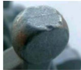
Fig. 2. Defect on the cast part
