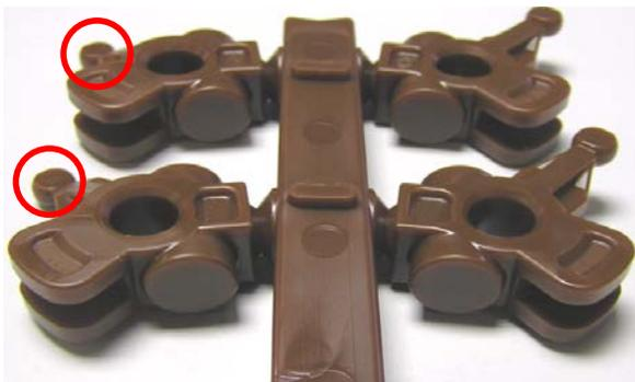
Fig.1. Structural defects on the wax tree
