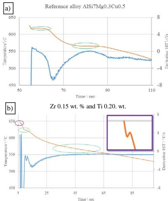
Fig. 5. a) Thermal analysis of the P reference alloy; b, E2 AlSi7Mg0.3Cu0.5Zr0.15 experimental alloy
