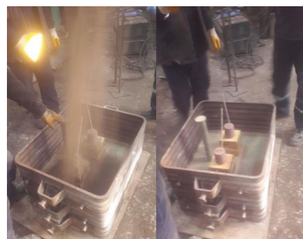
Fig. 3. Foundry workers are filling the drag than placing the core model
