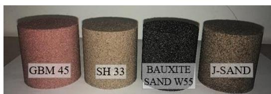
Fig. 4. Standard permeability test specimens
