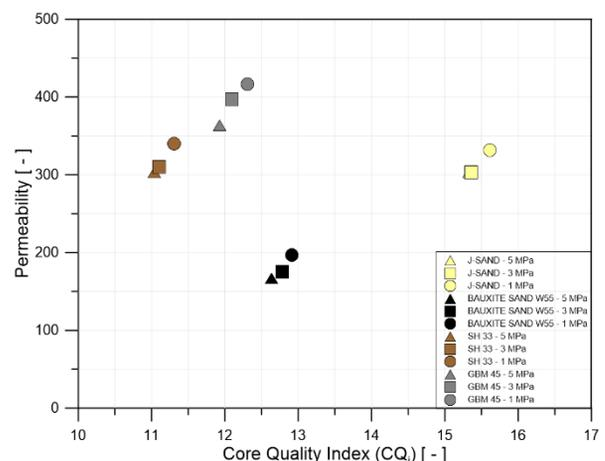
Fig. 7. The permeability test results as a function of  $CQ_i$  in the case of the investigated sands
