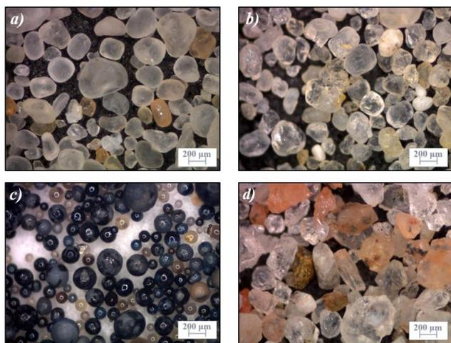
Fig. 1. Stereo microscopic images of the sands a) GBM 45, b) SH 33, c) Bauxite sand W55 and d) J-SAND at 20x magnification
