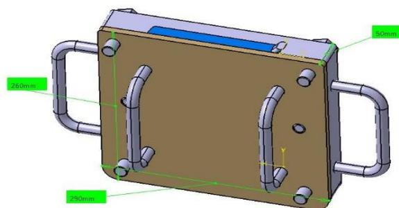
Fig. 4. Permanent Mold (290mm x 260mm x 50mm)
