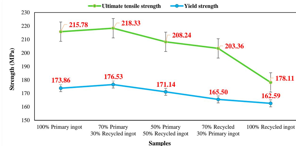
Fig. 7. Yield strength and ultimate tensile strength values of the samples
