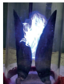
Photograph of the plasma taken during a GlidArc discharge in a cylindrical reactor with solid electrodes.
