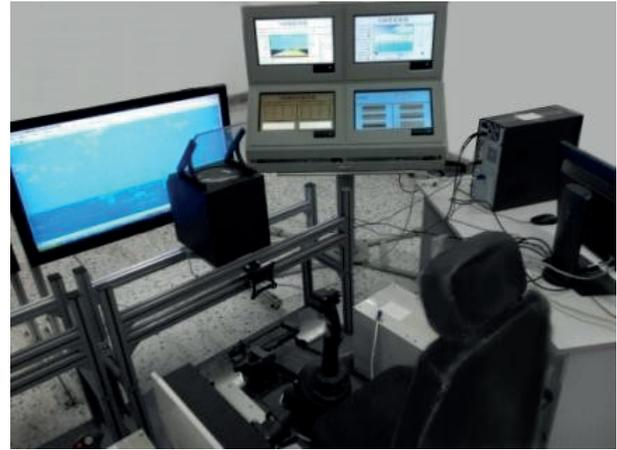
Fig. 10. Semi-physical landing simulation system
