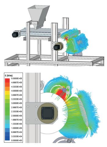
Fig. 4. The electric field distributions excited by the corona and deflection electrodes
