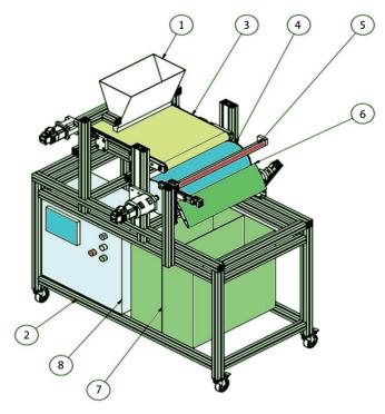
Fig. 3. Isometric view of the designed ES system: 1 – material feeder, 2 – aluminum frame, 3 – belt transporter, 4 – rotating drum, 5 – corona electrode, 6 – deflection electrode, 7 – material collectors, 8 – electrical cabinet
