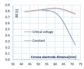
Fig. 8. The influence of the corona electrode position at constant and critical values of the voltage on the separation effectiveness coefficient
