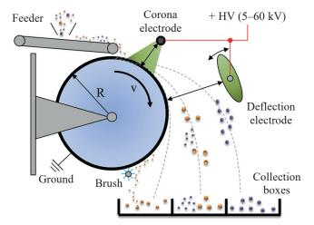
Fig. 2. Crucial elements and dimensions influencing the separation process in the typical configuration of a rotating electrode drum type separator
