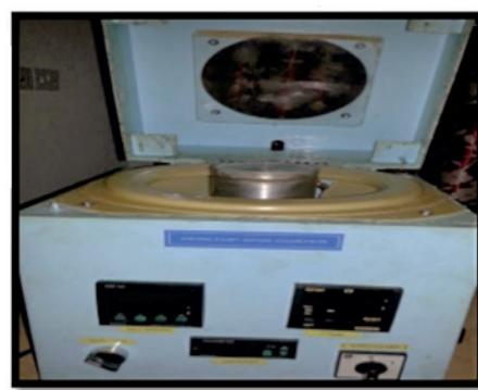
Fig. 1. Schematic and actual experimental spin coating device
