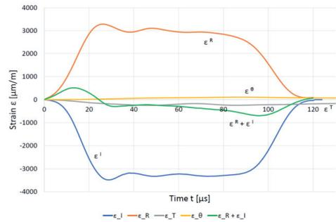
Fig. 9. List of dependencies of longitudinal strain of the bars ( $\varepsilon^I, \varepsilon^R, \varepsilon^T$ ) and the peripheral strain of the casing  $\varepsilon^\theta$  depending on the time  $t$  - sample  $w_2 = 4,6$  [%].
