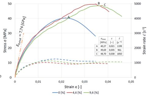
Fig. 15. Collective list of the dependence of stress - strain for the soils with less than total moisture ( $w < w_{sat}$ ).
