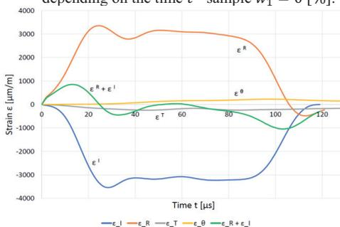
Fig. 10. List of dependencies of longitudinal strain of the bars ( $\varepsilon^I, \varepsilon^R, \varepsilon^T$ ) and the peripheral strain of the casing  $\varepsilon^\theta$  depending on the time  $t$  - sample  $w_3 = 9,6$  [%].
