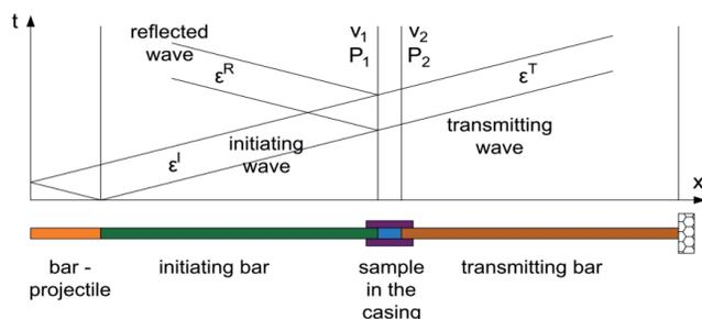
Fig 4. Wave chart illustrating the phenomenon of elastic wave propagation in a Split Hopkinson Pressure Bar.  $t$  - time,  $x$  - bar axis: bar-projectile and measuring bar,  $\varepsilon^I(t)$ ,  $\varepsilon^T(t)$ ,  $\varepsilon^R(t)$  - elastic strain of the measuring bars over time measured by strain gauges,  $P_1(t)$  and  $P_2(t)$  - dynamic forces at the ends of the tested sample,  $v_1(t)$  and  $v_2(t)$  - the velocity of the fronts of the measuring bars.
