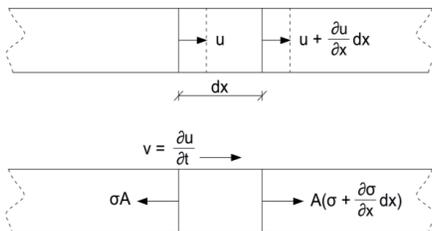
Fig. 6. Diagram of elastic wave propagation in a measuring bar [5].
