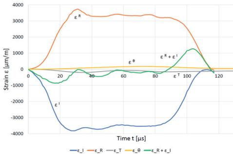
Fig. 8. List of dependencies of longitudinal strain of the bars ( $\varepsilon^I, \varepsilon^R, \varepsilon^T$ ) and the peripheral strain of the casing  $\varepsilon^\theta$  depending on the time  $t$  - sample  $w_1 = 0$  [%].
