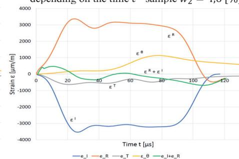
Fig. 11. List of dependencies of longitudinal strain of the bars ( $\varepsilon^I, \varepsilon^R, \varepsilon^T$ ) and the peripheral strain of the casing  $\varepsilon^\theta$  depending on the time  $t$  - sample  $w_4 = 14,6$  [%].
