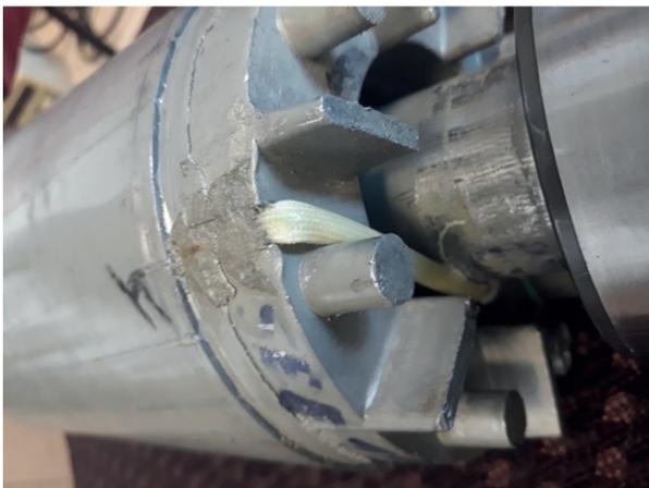
Fig. 6. Place of mounting of the thermocouple used to measure the temperature of a bar of the cage winding
