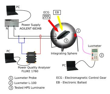
Fig. 1. Experimental setup for HPS luminaire with electromagnetic control gear and electronic ballast
