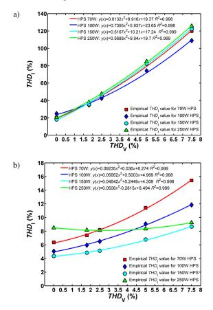
Fig. 3. The relationship between  $THD_I$  in a function of  $THD_V$ : (a) for HPS lamp with ECG, (b) for HPS lamp with EB
