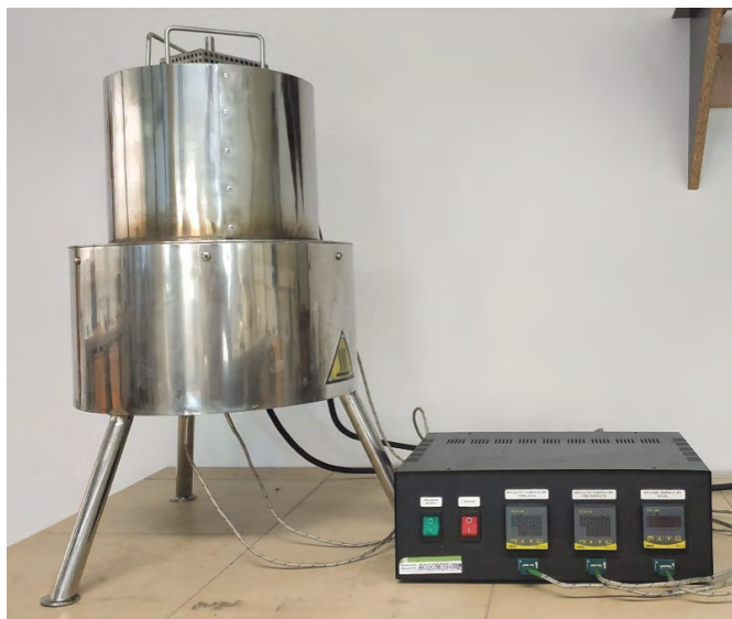
Photo 1. Two-chamber laboratory pyrolysis device
