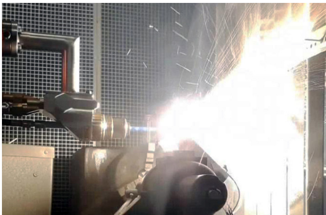
Fig. 1. Thermal test of Nb sample without coating
