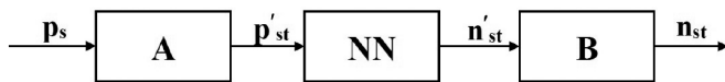
Fig. 10. Diagram of a mathematical model using neural networks, where [40]: p_s – input signal vector; p'_{st} is the standardized input signal vector; n'_{st} is the standardized output signal vector; n_{st} is the output signal vector, NN is the neural network and A and B are signal transformation matrices
