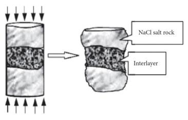
Fig. 12. Creep failure sketch map of bedded rock salt ([10] after [121])
