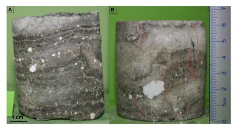
Fig. 4. The rock salt sample with claystone interlayers from the Łężkowice salt deposit: A-before test, B-after uniaxial compression test
