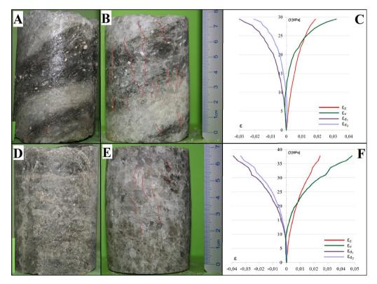
Fig. 8. Rock salt samples characterised by unevenly distributed impurities from the Łężkowice salt deposit
