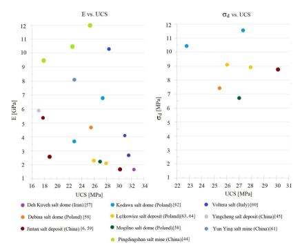
Fig. 2. The diversity of selected mechanical parameters: Young's modulus (*E*), uniaxial compressive strength (UCS) and stress at dilatancy threshold ( $\sigma_d$ ) in different rock salt deposits [6,44,45,57-64]
