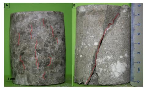
Fig. 6. Comparison between failure mode of rock salt and salty claystone from the Łężkowice salt deposit: A – tensile-shear failure mode of rock salt, B – single shear crack in salty claystone
