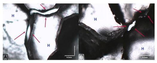
Fig. 3. The cracks at the crystal boundaries in a pink rock salt samples (double polished sections about 1-3 mm thick, parallel nicols) from the Kłodawa salt dome after uniaxial compression tests: H – halite, cracks are marked by red arrows
