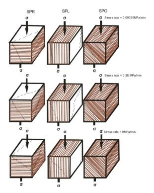
Fig. 5. Crack patterns developed in samples deformed perpendicular, parallel, and oblique to bedding [43]
