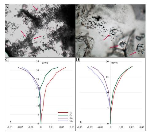
Fig. 7. The of samples rock salt from the LGOM characterise by different mechanical properties: A – microscopic image of sample with high UCS, B – microscopic image of sample with low UCS, C – stress-strain characteristic of sample with high UCS, D – stress-strain characteristic of sample with low UCS ([73] modified)
