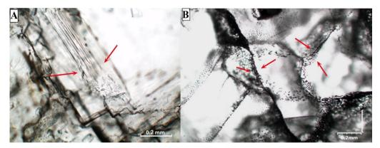
Fig. 9. Fluid inclusion plains at halite grain boundaries: A - rock salt from LGOM (double polished sections about 1-3 mm thick, parallel nicols) rock salt, B - pink rock salt from the Kłodawa salt dome
