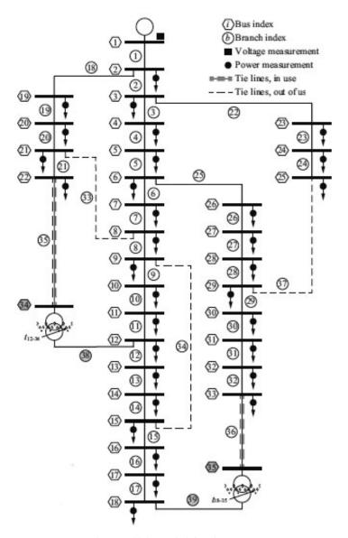
Fig. 8. IEEE 33-bus radial distribution system
