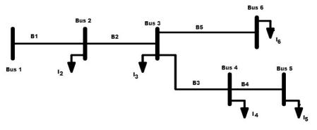
Fig. 1. Simple distribution system
