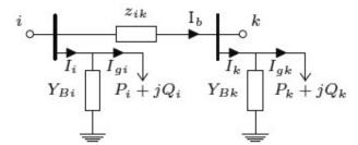
Fig. 6. Pseudo Pi-equivalent model of the smart transformer
