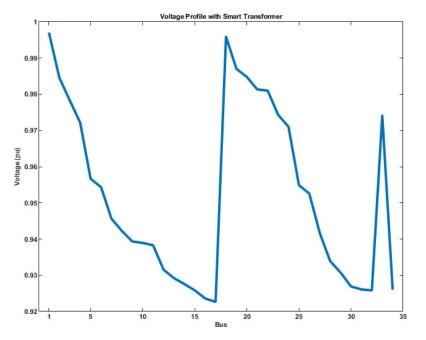
Fig. 10. Voltage profile with smart transformer for IEEE 33-bus system
