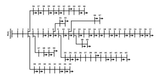
Fig. 7. Single line diagram of IEEE 69-bus network
