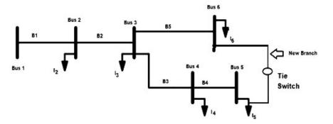
Fig. 2. Simple distribution system with one loop
