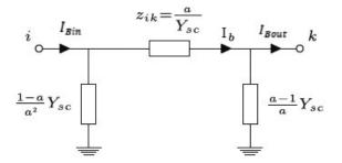
Fig. 5. Pi-equivalent model of the smart transformer
