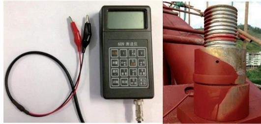
(a) Anchor cable reader (b) Rope meter
