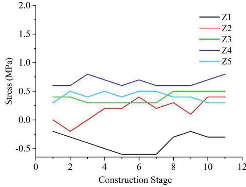
Fig. 9. Z direction stress diagram of key section in each construction stage (MPa)
