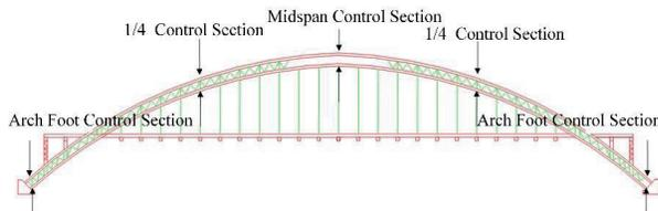
Fig. 5. Stress control section layout
