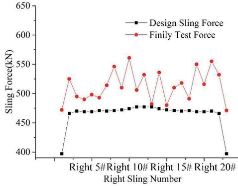
Fig. 15. Comparison diagram of cable force before and after replacement of right cable
