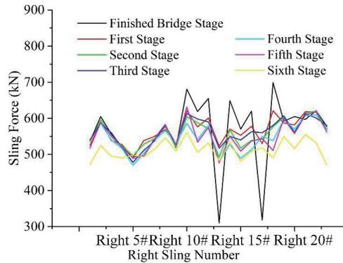
Fig. 14. Sling force of the right sling at each stage
