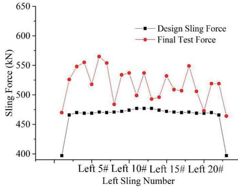
Fig. 16. Comparison diagram of cable force before and after replacement of left cable
