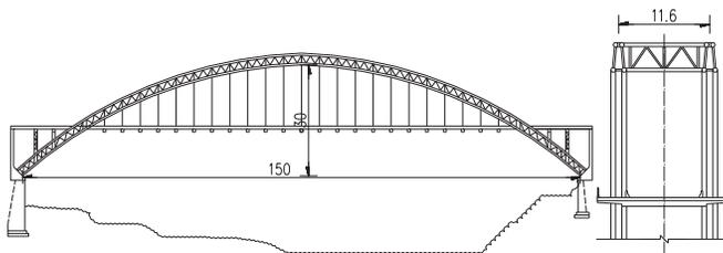
Fig. 2. Elevation and cross-sectional drawing (m)
