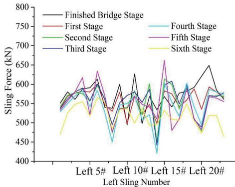
Fig. 13. Sling force at each stage of left sling
