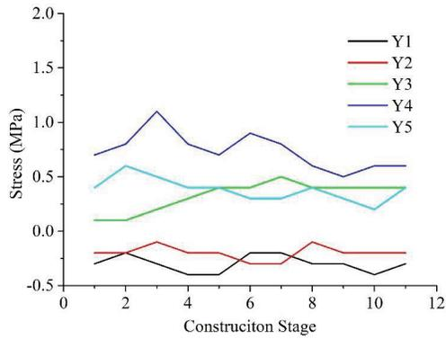
Fig. 8. Y-direction stress diagram of key section at each construction stage (MPa)
