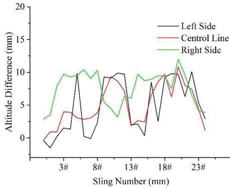
Fig. 10. Change elevation difference between left side, center line and right side of bridge before and after
