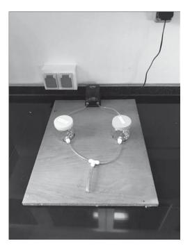
Fig. 1. Y-tube olfactometer used in the study
