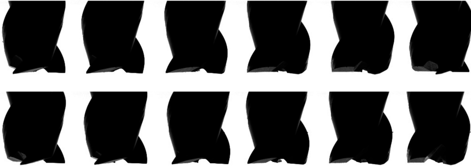
Fig. 5. A sequence of end mill images acquired at the spindle speed of 50 r/min.
