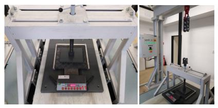
Fig. 4. Test of the axle weighing instrument in the Laboratory for testing of weighing instruments of Slovak Legal Metrology.
