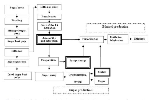
Fig. 4. Technological scheme for the production of sugar and bioethanol from sugar beet at a sugar beets processing plant Source: formed by the authors according to previous studies (Kaletnik and Pryshliak 2013; Pryshliak 2014)
