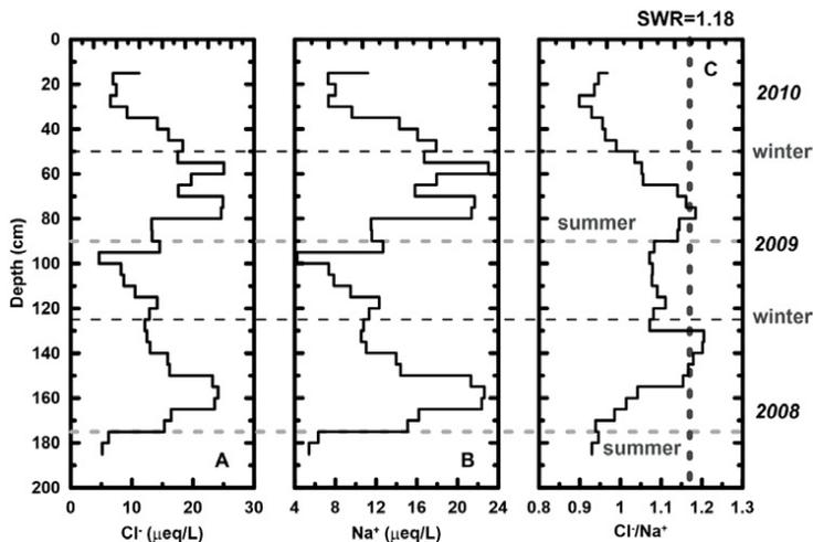
Fig. 4. Vertical profiles of  $\text{Cl}^-$  (A),  $\text{Na}^+$  (B) and the  $\text{Cl}^-/\text{Na}^+$  ratio (C). The dashed line represents the  $\text{Cl}^-/\text{Na}^+$  ratio in the Sea Water Ratio (SWR, 1.18).
