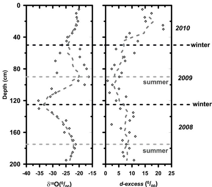
Fig. 3. Vertical profiles of stable water isotopes ( $\delta^{18}\text{O}$  in the left and deuterium excess in the right, respectively). Summer and winter in the snowpit were defined from the maximum and minimum values of the stable water isotopes, respectively.
