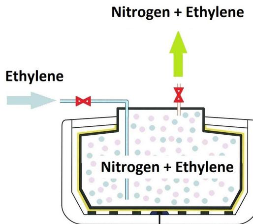
Figure 3: Removing the nitrogen by total mixing of nitrogen and ethylene.
