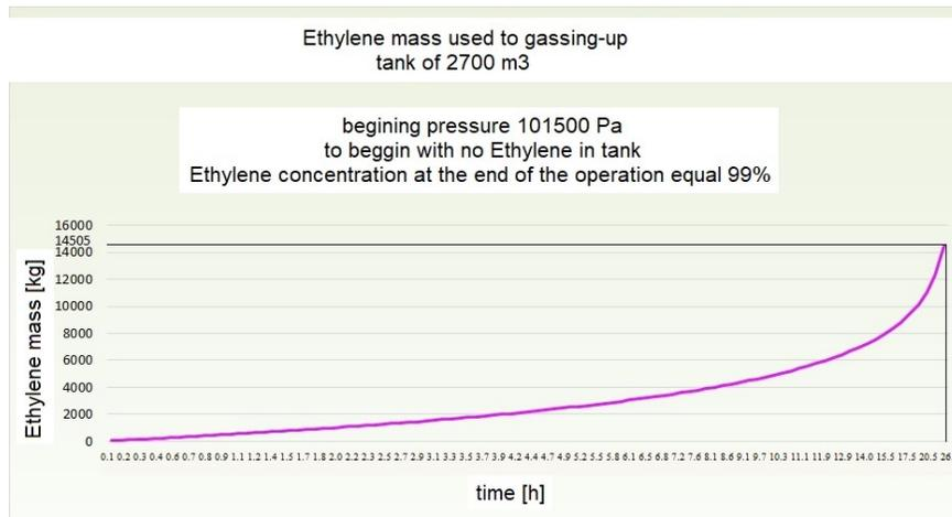
Figure 7: The amount of ethylene used to carry out the gassing-up process as a function of time (without increasing the tank pressure by introducing the ethylene vapour).
