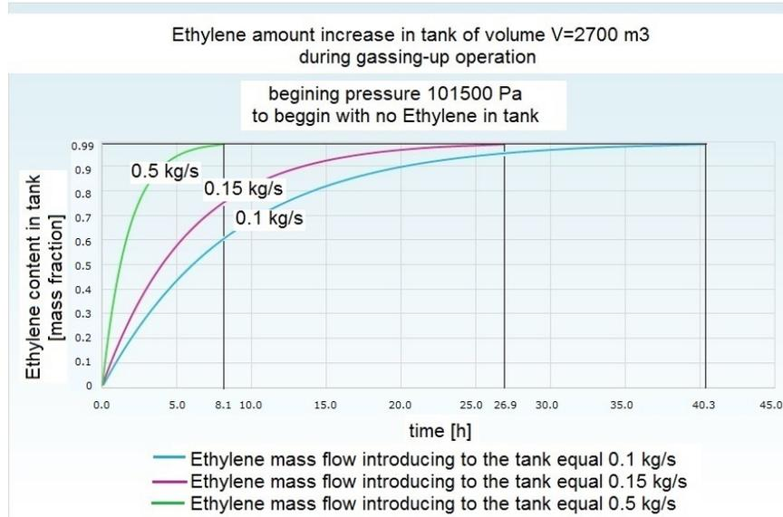
Figure 5: Increasing the amount of ethylene in the tank as a function of gassing-up time for different mass flow values (without increasing the tank pressure by introducing the ethylene vapour).
