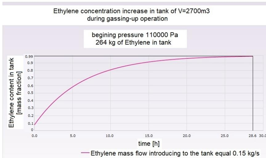
Figure 9: Ethylene amount increase in tank as a function of time (after introducing 264 kg of ethylene to increase the tank pressure).
