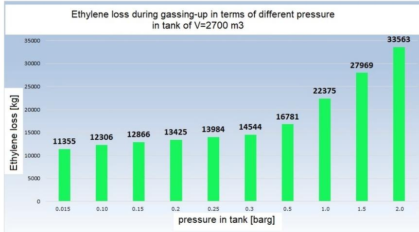
Figure 8: Ethylene loss during the tank gassing-up relative to different tank pressures, at which the process is carried out.
