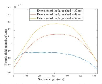
Fig. 8. Electric field distribution of icing insulators with different extension differences of the shed
