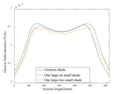
Fig. 6. Electric field distribution of icing insulators with different shed structures
