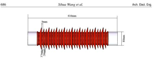
Fig. 9. Structure diagram of optimized insulator
