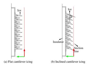
Fig. 3. Two-dimensional cantilever icing insulators
