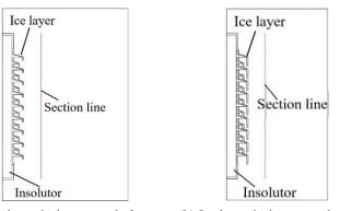
(a) Ice layer thickness equals 3 mm, icicle length equals 13 mm
