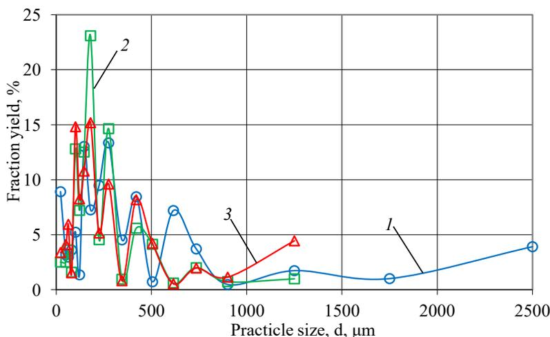
Fig. 2. Differential distribution curves of grinded amber ( $q \geq 0.95$ ;  $n = 3$ ): 1 – aqueous medium, 250 kJ; 2 – alcohol medium, 125 kJ; 3 – alcohol medium, 250 kJ
