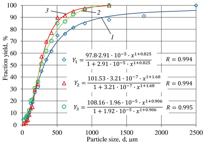
Fig. 3. Integral distribution curves of grinded amber ( $q \geq 0.95$ ;  $n = 3$ ): 1 – aqueous medium, 250 kJ; 2 – alcohol medium, 125 kJ; 3 – alcohol medium, 250 kJ
