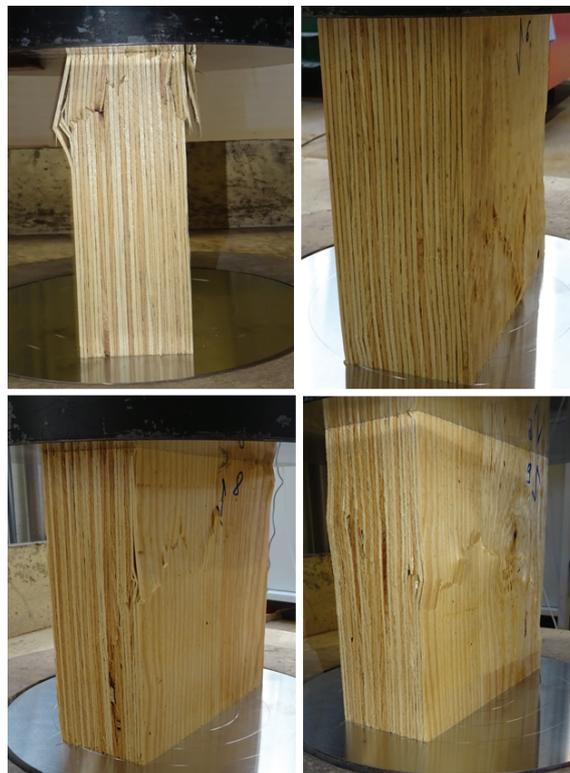
Fig. 10. The failure modes of the LVL R panels in the compressive tests
