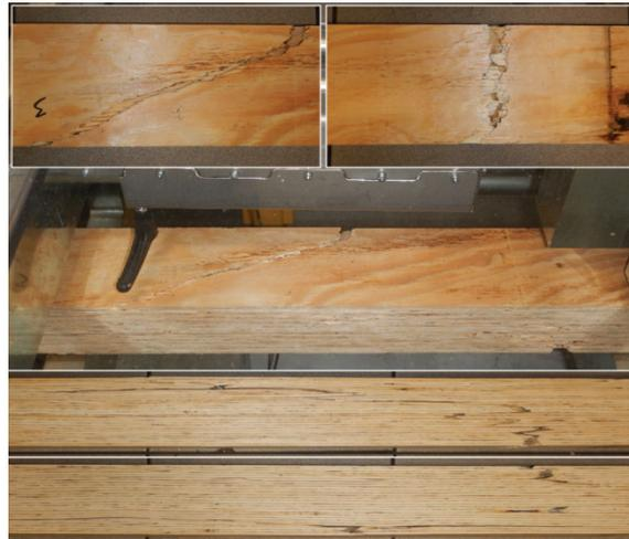
Fig. 9. The failure mode of the LVL R panel in the tensile test
