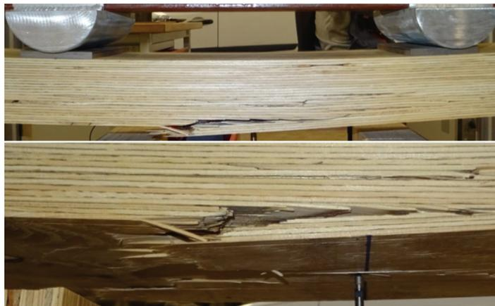
Fig. 13. The failure mode of the LVL R panel from the bending test
