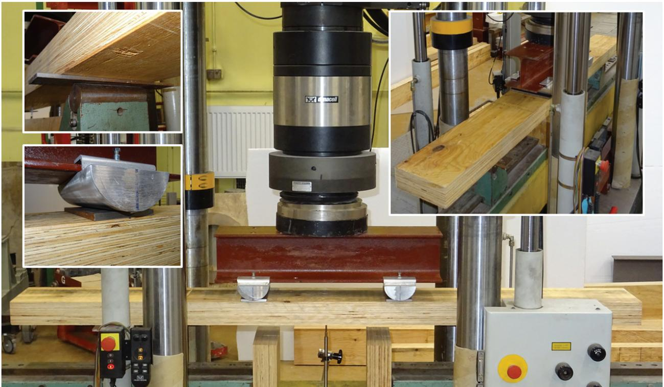
Fig. 3. The LVL R panel investigated in the four-point bending test
