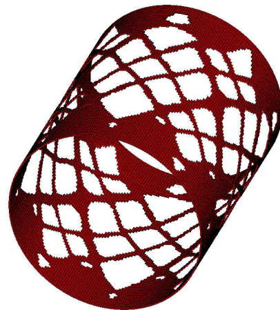
Fig. 32. Results: The final topology of the cylindrical shell
