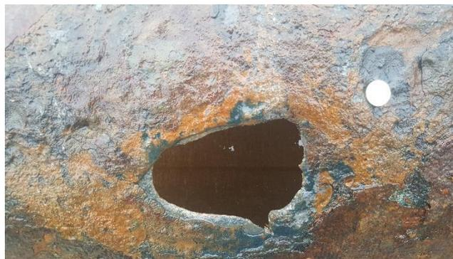
Fig. 4. Corrosion damage of water pipe as a result of stray currents
