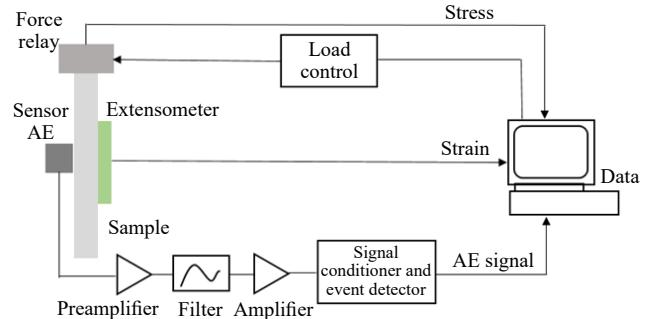
Fig. 4. Diagram of the measuring station.
