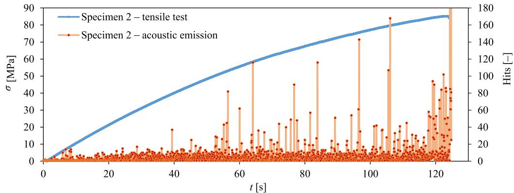
Fig. 7. Graph of stress and number of AE hits as a function of time for a selected sample with 10% recyclate content.
