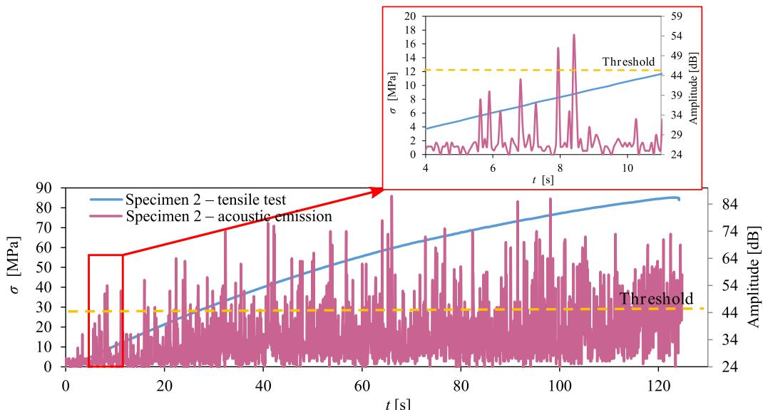
Fig. 9. Graph of stress and amplitude of acoustic emission signals as a function of time for a sample with 10% polyester-glass recyclate content.
