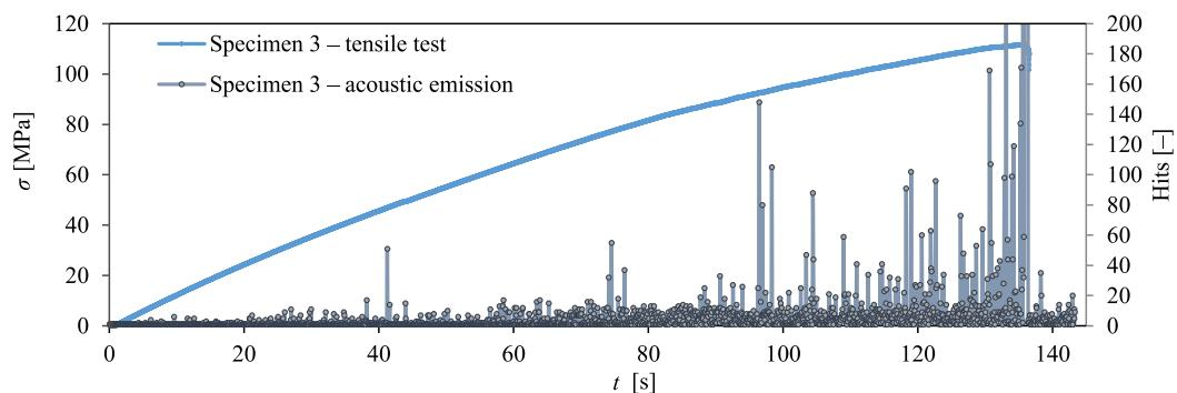
Fig. 6. Graph of stress and number of AE hits, as a function of time for a selected sample without recyclate.
