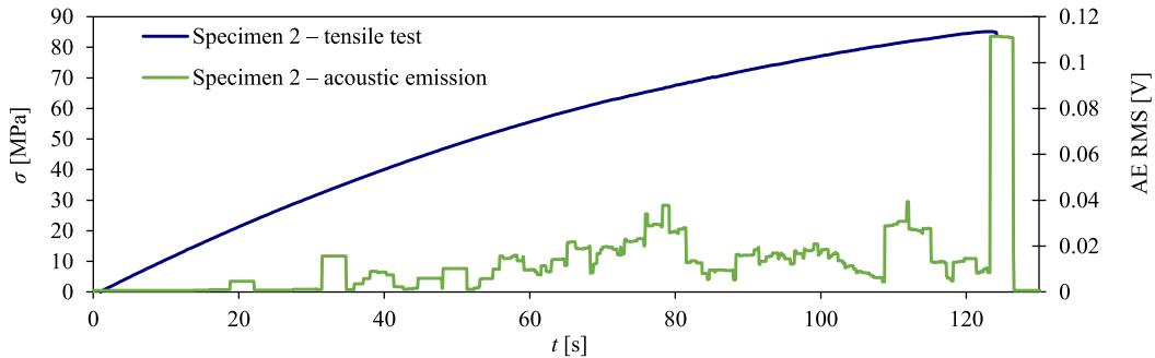
Fig. 12. Stress and RMS graph as a function of time for a sample with 10% polyester-glass recyclate content.
