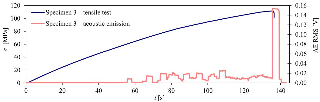
Fig. 11. Stress and RMS graph as a function of time for a sample without recyclate.
