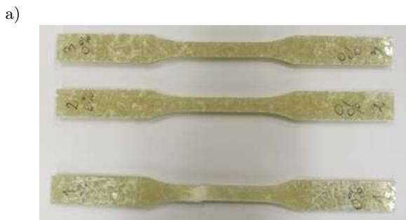
Fig. 3. View of specimens used in research: a) composite without recyclate, b) composite with 10% of recyclate.
