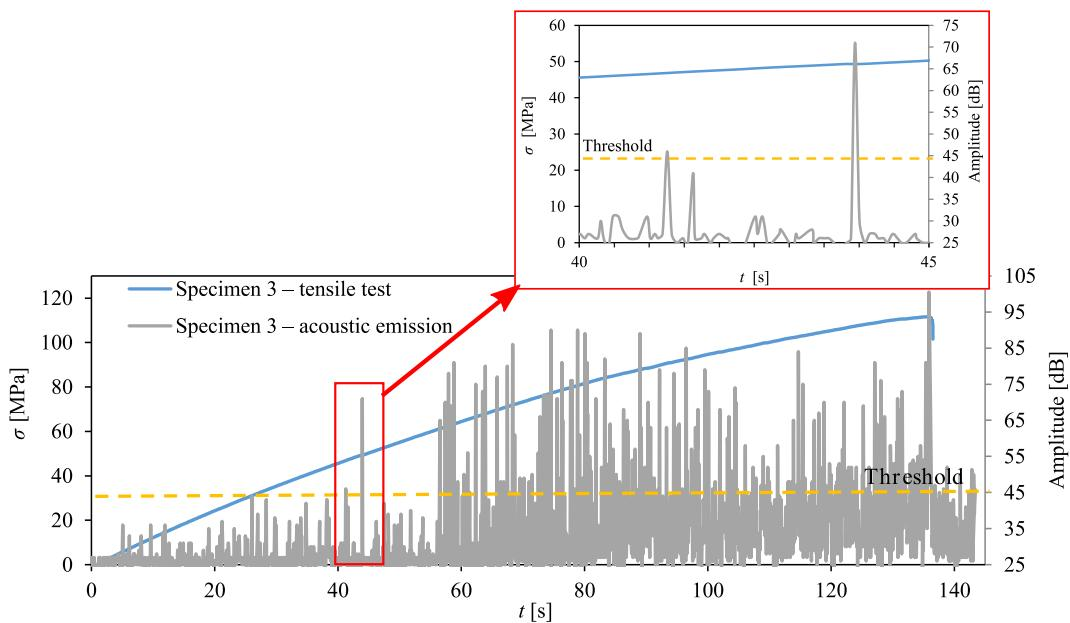
Fig. 8. Graph of stress and amplitude of acoustic emission signals as a function of time for a sample without recyclate.
