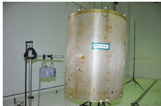
Fig. 6. The cylinder being excited by a shaker.
